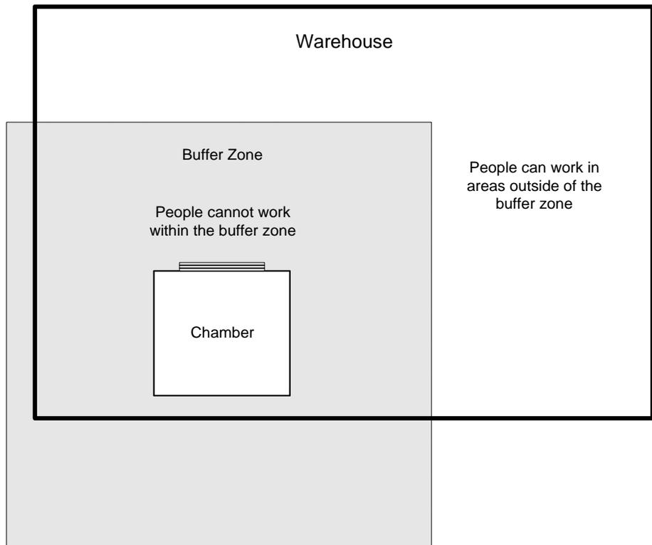
Vacuum chamber - Since a vacuum chamber is under negative pressure, methyl bromide cannot be released from any leaks. NOTE: buffer zones still apply.
